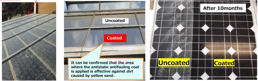
In the desert area where it doesn't rain like the panel in the left picture above, the air is a dry and the sand is charged and easy to adhere. Solar panel glass is required to have a surface that is difficult to adhere.
