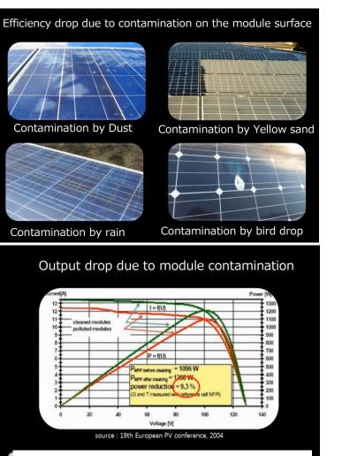
Up to 9.3% reduction in power generation output due to contamination
