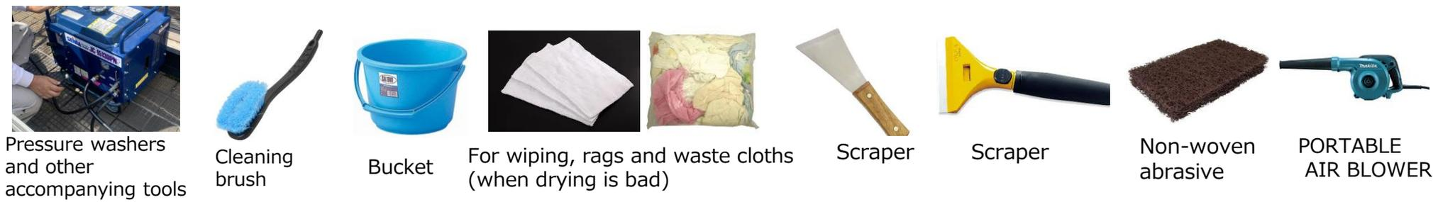
Pressure washers and other accompanying tools    Cleaning brush    Bucket    For wiping, rags and waste cloths (when drying is bad)    Scraper    Scraper    Non-woven abrasive    PORTABLE AIR BLOWER
